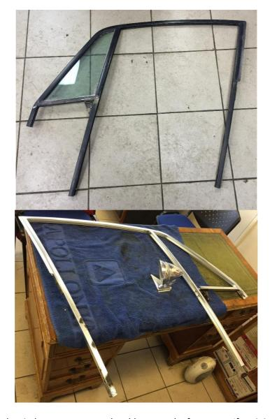
You may need a little window movement to be able to get the frame out. If so, it is a simple-enough matter to de-couple the regulator assembly from the motor. Then you'll be able to manually adjust the window position.
