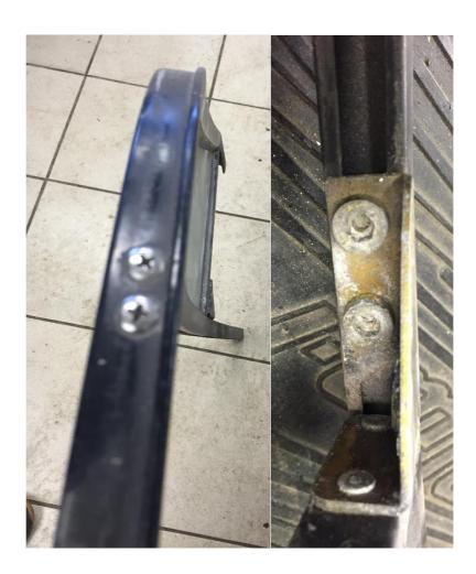
5. The new mirror just tucks into the quarter light glass, and is retained by the seal. When you refit the glass back into the door frame and add the vertical support bar, it is all held firmly together.
